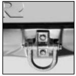
Your vehicle is equipped with recovery loops at the front and rear. You may need to use them if you're stuck off-road and need to be pulled to some place where you can continue driving.
